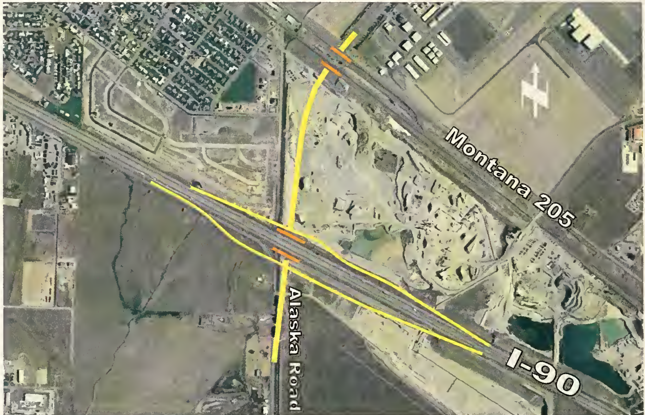
Figure 2-3 Compressed Diamond Interchange
